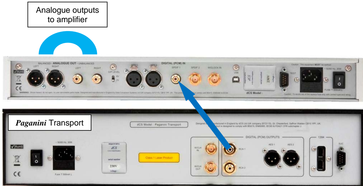
Figure 2 – Connecting an SPDIF interface.
